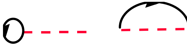
Figure 29-5 Pieces of diagrams for which lead to equal-time Green’s functions and for which it is necessary to specify how the \tau \rightarrow 0 limit is taken.
