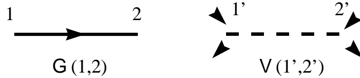
Figure 5-1 Basic building blocks of Feynman diagrams for the electron gas.
