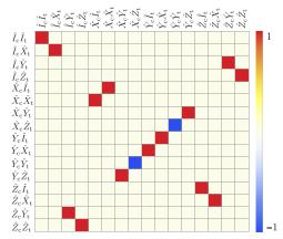
**Fig. 3. Pauli transfer matrix of the CX gate.** The transfer matrix is obtained by simulating the Hamiltonian in Eq. 26 with  $\alpha = \beta = 2$ ,  $\phi(t) = \pi t/T$ , and T = 10/K. The infidelity of this CX operation with respect to an ideal two-level CX is  $9.3 \times 10^{-7}$  and results from nonadiabatic transitions due to finite *KT*.
