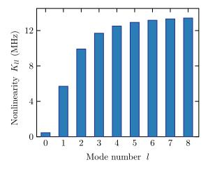
FIG. 8. Calculated self-Kerr shifts per photon  $K_{II}$  for different modes of the Josephson junction array described in Sec. I.
