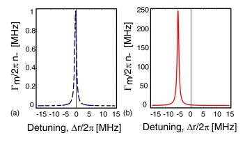
FIG. 6. (Color online) Dephasing rate  $\Gamma_{\rm m}$  as a function of the detuning  $\Delta_r$  between the bare resonator frequency  $\omega_r$  and the measurement drive frequency  $\omega_d$  for fixed  $\bar{n}_-$ =2. (a) Experimental parameters given in Sec. III. (b) Same as (a) but with a larger cavity pull  $\chi/2\pi=5$  MHz.
