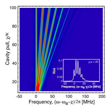
FIG. 8. (Color online) Spectrum  $S(\omega)$  as a function of the cavity pull  $\chi/\kappa$ . The detuning is  $\Delta_r = \chi$  such that the cavity is always driven at the dressed frequency  $\omega_r - \chi$ . Other parameter values are the same as in Fig. 7. Inset: Spectrum at  $\chi/\kappa = 20$ . At this experimentally realistic value of the cavity pull, the number splitting should be resolvable.
