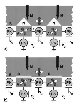
FIG. 1. (a) Superconducting DND qubits: A, B are *d*-wave superconductors, *N* normal conductor, PK parity key, *M* scanning tip,  $\Omega$  the mismatch angle between the lattices of *A* and *B*. The cut in *B* is here along (110) and (110) directions. Positive lobes of *d*-wave order parameter are shaded. Two qubits are shown. (b) Version of (a) using grain boundary (*G*) junctions.
