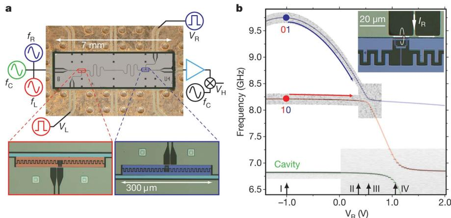
**Figure 1 | Two-qubit cQED device, and cavity/qubit characterization.**
