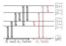
FIG. 2. (Color online) Transitions driven by noise. X and  $\sigma_x$  baths can only generate transitions between states of different parity. The  $\sigma_z$  bath can generate transitions between any pair of levels of same parity.
