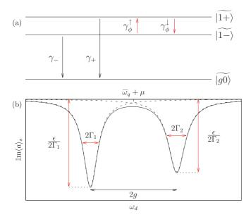
FIG. 4. (Color online) Vacuum Rabi splitting. (a) Transition rates involved in the perturbative calculation in the three-level approximation. (b) Schematic plot of  $\text{Im}\langle a \rangle_s$  as a function of  $\omega_d$ . In general, the result is not symmetric.
