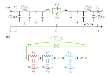
FIG. 2. (Color online) (a) Discretized representation of a transmission-line resonator capacitively coupled to input and output ports and with a Josephson junction interrupting the center conductor at position  $x_J$ . (b) Lumped element representation of the transmission line + junction. The normal modes of the resonator, dressed by the junction's capacitance and linear inductance, are represented by *LC* circuits biasing the junction's nonlinear inductance (spiderlike symbol).
