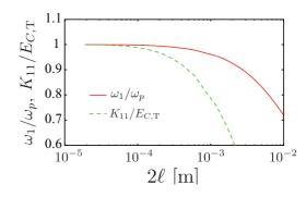
FIG. 9. (Color online)  $\omega_1/\omega_p$  (full red line) and  $K_{11}/E_{C,T}$  (green dashed line) vs total resonator length  $2\ell$ . For very short lengths, the circuit essentially behaves as a transmon of frequency  $\hbar\omega_p = \sqrt{8E_{C,T}E_J}$  and anharmonicity  $E_{C,T} = e^2/[2(2\ell C^0/4 + C_J)]$ .
