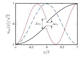
FIG. 3. (Color online) Typical example of the first three normal mode envelopes of a resonator with a Josephson junction at  $x_J = 0$ .
