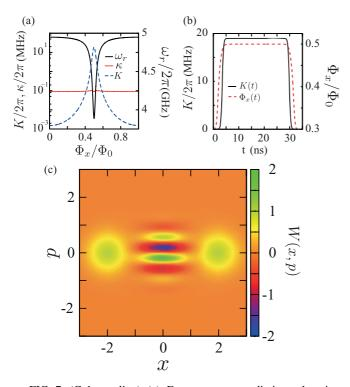
FIG. 7. (Color online) (a) Frequency  $\omega_r$ , radiative relaxation rate  $\kappa$ , and self-Kerr coefficient *K* of the first mode as a function of external flux. (b) Pulse shape of the external flux and Kerr coefficient as a function of time for Schrödinger cat state generation. (c) Density plot of the numerically obtained resonator Wigner function immediately after the flux pulse acting on an initially coherent state  $|\alpha = 2\rangle$ . The device parameters are given in text.
