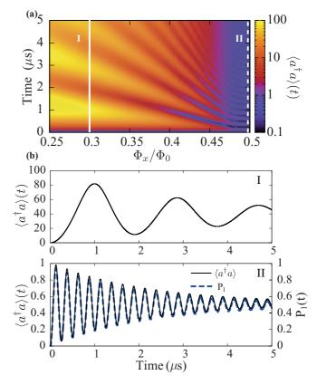
FIG. 8. (Color online) (a) Density plot of the average number of photons as a function of time and external flux in the presence of an external drive of amplitude  $\epsilon/2\pi = 2$  MHz and of frequency  $\omega_d = \omega_r - K/2$ . (b) Line cuts for the values of flux indicated by I and II in panel (a) and corresponding, respectively, to  $K/\kappa \sim 1/25$  and  $\sim 200$ .
