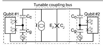
FIG. 3. A pair of charge-phase qubits capacitively coupled to a CBJJ.
