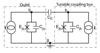
FIG. 1. A pair of capacitively coupled CBJJ qubits.
