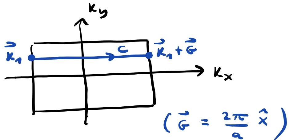
$$\gamma_m = \oint_C \vec{A}_m(\vec{k}) \cdot d\vec{k} - i \ln \left[ \langle u_{\vec{k}_1, m} | u_{\vec{k}_1 + \vec{G}, m} \rangle \right]$$
