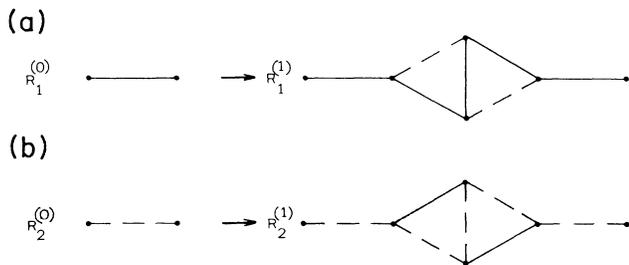
FIG. 1. Patterns which are concomitantly iterated to form a hierarchical structure. Solid lines represent resistance with value  $R_1^{(0)}$ , and dashed lines, resistances with value  $R_2^{(0)}$ . The pattern (a) becomes a resistance  $R_1^{(1)}$  for the next level of iteration, and the pattern (b) becomes a resistance  $R_2^{(1)}$ .
