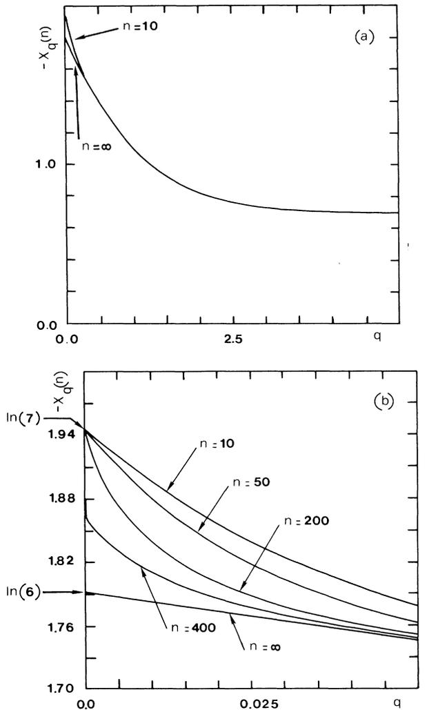
FIG. 2. Exponents, as defined by Eqs. (1) and (6), for the moments of the current distribution in the lattice of Fig. 1. (a) Curve for various values of the level of iteration (coarse  $q$  scale). (b) Enlargement of the  $q$  scale near the origin. ( $\epsilon_0 = 10^{-6}$ .)
