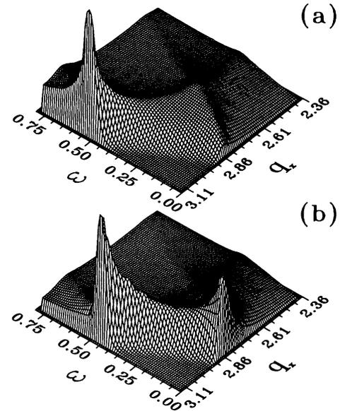
FIG. 2. The imaginary part of the susceptibility at finite  $U$  for  $x = 0.14$ ,  $t' = 0$ ; (a)  $U/U_c = 0.75$  and (b)  $U/U_c = 0.975$  for a  $4000 \times 4000$  lattice. The overdamped mode softens as  $U$  approaches the ISDW instability at a renormalized value of  $U_c = 2$ . The peak in the intensity as a function of wave vector decreases as the frequency  $\omega$  increases, as long as  $\omega$  is larger than the resonance frequency.
