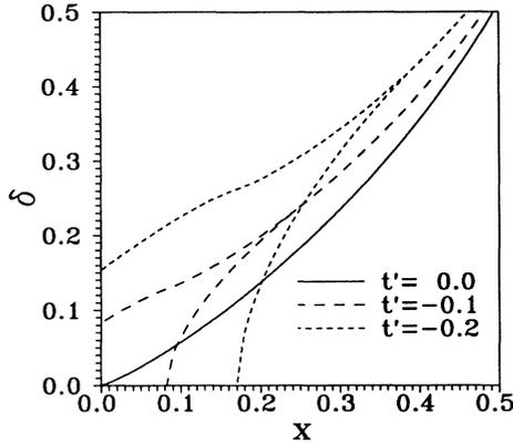
FIG. 1. Peak displacement  $\delta$  vs dopant concentration  $x$  (decreasing  $\mu$ ) for three values of  $t'$  (0,  $-0.1$ , and  $-0.2$ ) at low temperatures and low frequencies ( $T, \omega \ll 2|\mu|$ ), as predicted by GRPA with renormalized  $U$ .
