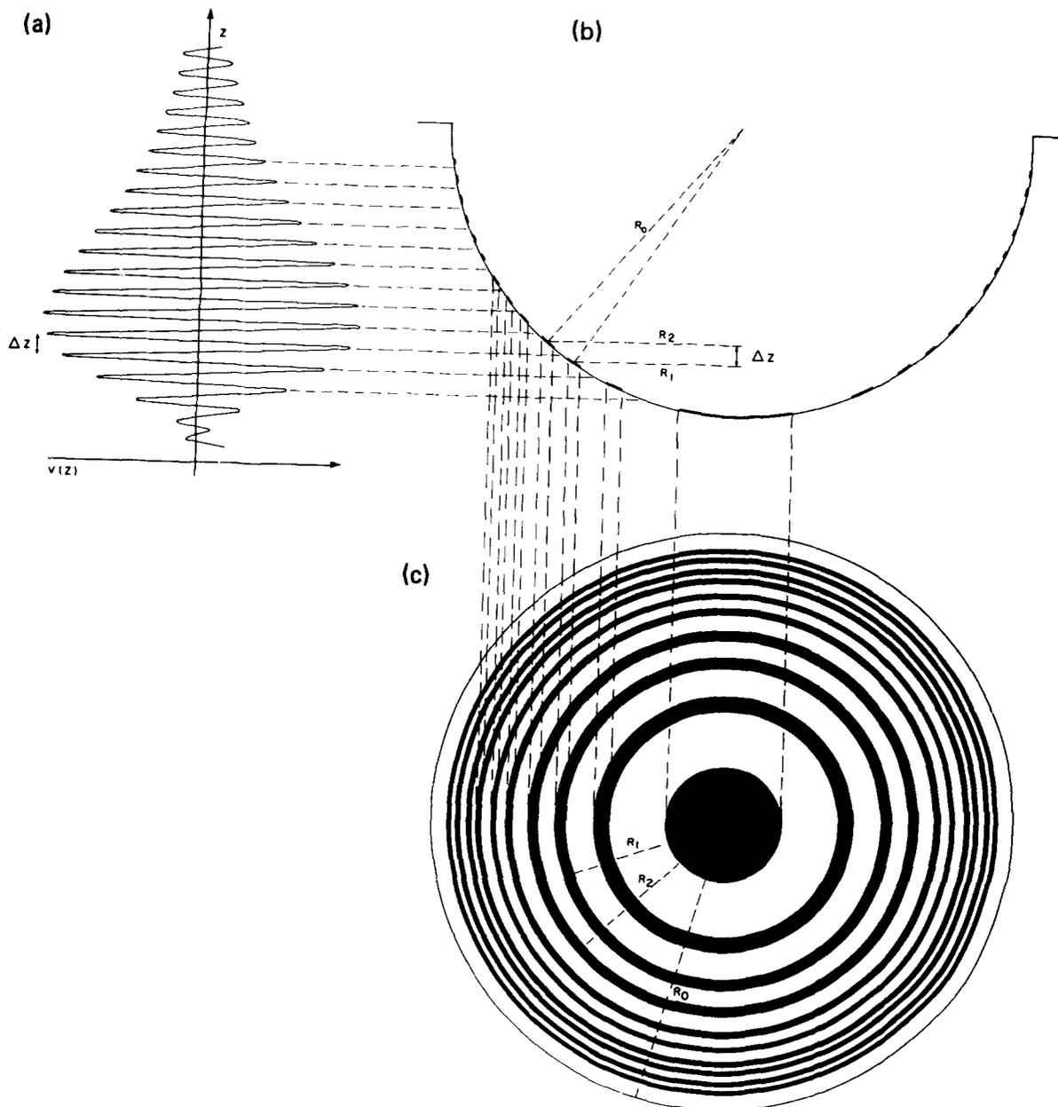
FIG. 5. AMS imaging of a concave spherical surface at 150 MHz. (a) One-dimensional AMS obtained on a concave spherical surface, (b) scanning of one line over the concave spherical surface, (c) complete acoustic image: when the lens-to-surface spacing is changed by  $\Delta z$  equal to the effective wavelength, a bright or dark ring appears. By measuring  $R_1$ ,  $R_2$ , etc., the radii of the rings, one can reconstruct the profile of the nonplanar surface.
