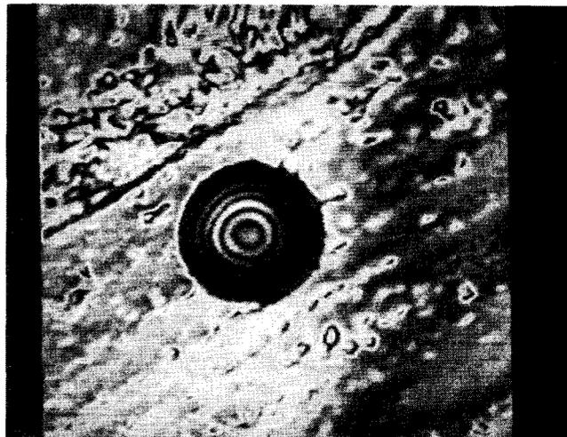
FIG. 4. Acoustic image of a spherical cavity ground and polished in an  $\text{Al}_2\text{O}_3$  (c) buffer.  $R_0 = 80 \mu\text{m}$ ,  $f = 150 \text{ MHz}$ . Field of view  $512 \times 512 \mu\text{m}^2$ .
