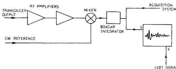
FIG. 1. Experimental setup for AMS recording and imaging.
