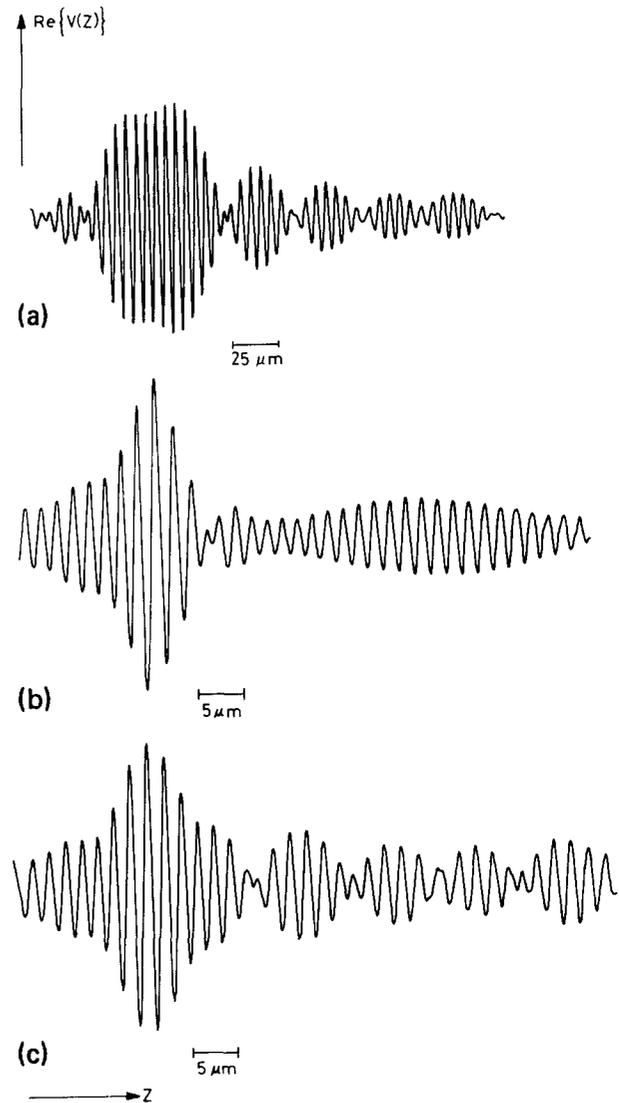
FIG. 2. Acoustic material signatures (AMS). (a) Duralumin planar surface at 150 MHz, (b)  $\text{Al}_2\text{O}_3$  (c) planar surface-gold film (1500 Å) at 450 MHz, (c)  $\text{Al}_2\text{O}_3$  (c) planar surface-gold film (1500 Å)-ZnO film (3.5  $\mu\text{m}$ ) at 450 MHz.
