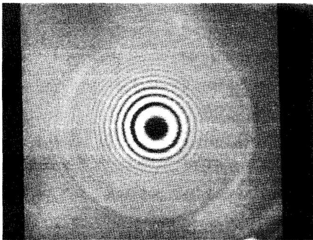
FIG. 3. Acoustic image of a spherical cavity ground and polished in an  $\text{Al}_2\text{O}_3$  (c) buffer.  $R_0 \approx 215 \mu\text{m}$ ,  $f = 150 \text{ MHz}$ . Field of view  $512 \times 515 \mu\text{m}^2$ .
