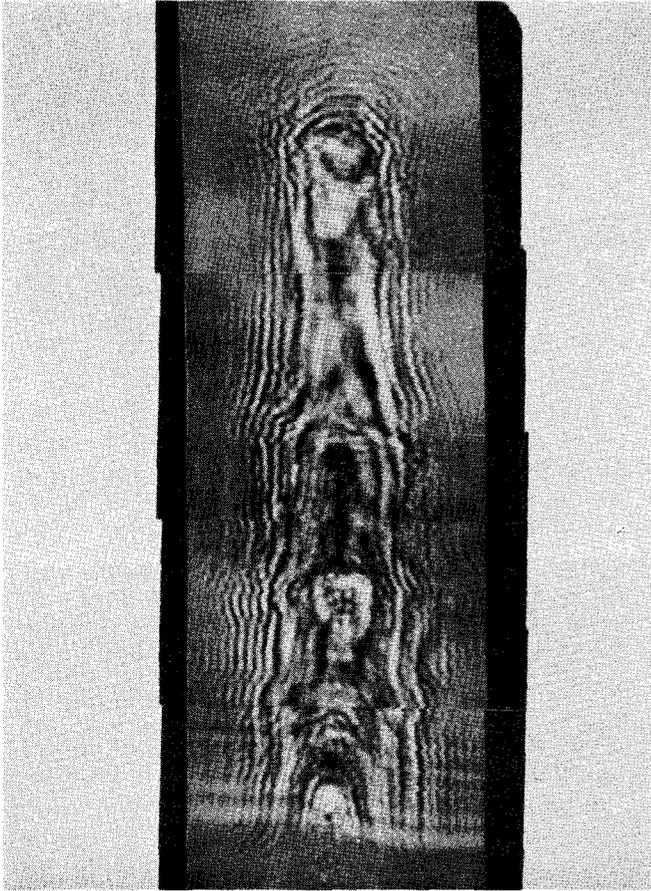
FIG. 6. AMS imaging of a subsurface defect at 150 MHz: drilled hole under the surface of a duralumin planar surface. Diameter  $\approx 475 \mu\text{m}$ , depth  $\approx 90 \mu\text{m}$ . Field of view  $0.5 \times 1.5 \text{ mm}^2$ .
