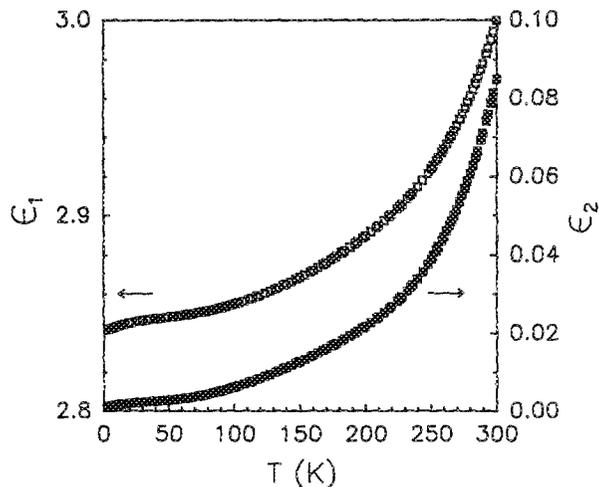
FIG. 1. Complex dielectric function  $\epsilon_1 - j\epsilon_2$  of Stycastr 1266 resin at 16.8 GHz as a function of temperature.  $\epsilon_1$ : dielectric constant;  $\epsilon_2$ : dissipation factor.
