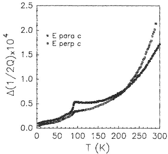
FIG. 2. Relative microwave absorption  $\Delta(1/2Q)$  in a pure rf electric field as a function of temperature for two field orientations.
