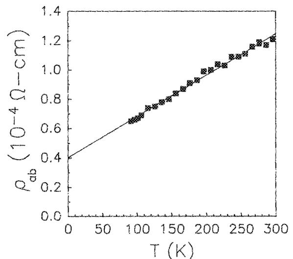
FIG. 4. Resistivity in the  $a$ - $b$  plane as deduced from the microwave absorption obtained with  $H_r$  parallel to  $c$ . A linear regression (continuous line) gives  $\rho_{ab} = 40 \mu\Omega \text{ cm} + 0.282 \mu\Omega \text{ cm/k T}$ .
