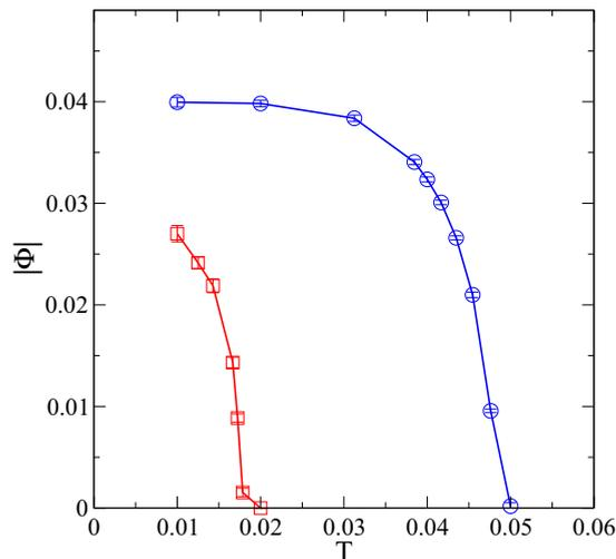
FIG. 3. (Color online)  $d$ -wave superconducting order parameter  $\Phi$  as a function of temperature  $T$  for  $U = 9.0$  and  $\delta = 0.04$ , with and without four-operator updates (circles and squares, respectively).
