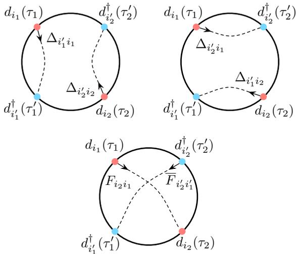
FIG. 1. (Color online) Diagrams contributing to the weight of a second-order configuration, cf. Eq. (8). The bold black circle represents the trace with the impurity operators, connected in all different ways by the hybridization function.
