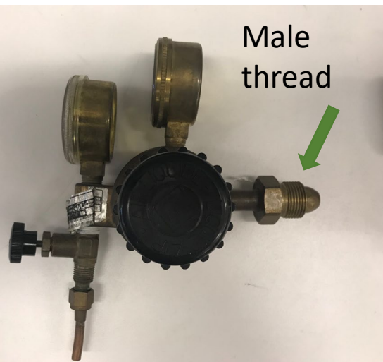
Regulator for inert gasses ( N_2 , Ar, He).
