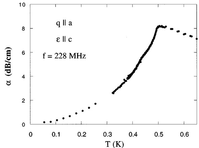
FIG. 2. Transverse ultrasonic attenuation  $\alpha_{ac}$  for propagation along  $\hat{a}$  and polarization along  $\hat{c}$ . The attenuation drops much more quickly than  $\alpha_{ab}$ , reflecting the insensitivity of  $\alpha_{ac}$  to quasiparticles in the basal plane.
