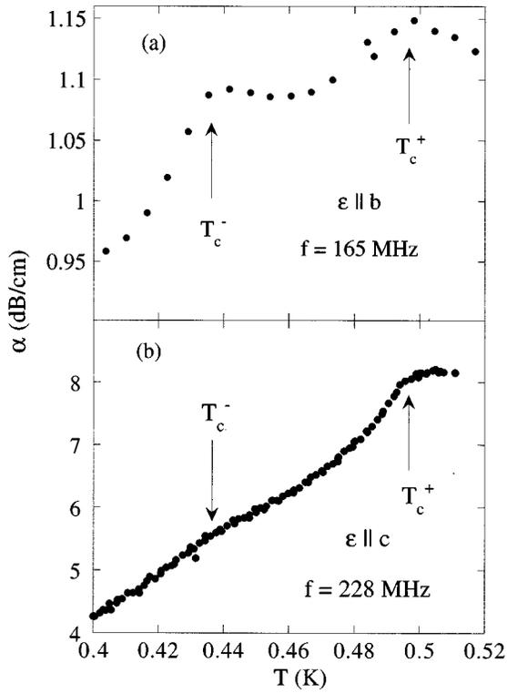
FIG. 3. (a) Detail of  $\alpha_{ab}$  in the *A* phase. After a drop at  $T_c^-$ , the attenuation reaches a plateau before dropping sharply on entering the *B* phase. This behavior reflects a larger quasiparticle density in the *A* than in the *B* phase. The arrows designate  $T_c^-$  and  $T_c^+$  as determined from longitudinal sound velocity data Ref. 10. (b) Detail of  $\alpha_{ac}$  in the *A* phase. The onset of the *B* phase is evident as a small “bump” near  $T_c^- = 435$  mK.
