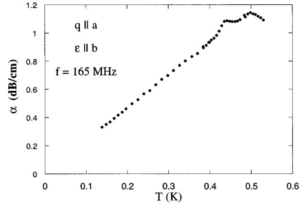
FIG. 1. Transverse ultrasonic attenuation  $\alpha_{ab}$  for propagation along  $\hat{a}$  and polarization along  $\hat{b}$ . The low-temperature attenuation shows no curvature down to 130 mK.
