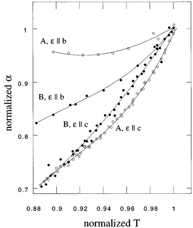
FIG. 4. Transverse attenuation data for both polarizations normalized to the value of the attenuation at  $T_c^+$  and  $T_c^-$  as a function of  $T/T_c^{\pm}$ . This choice of normalization allows us to compare the attenuation in the *A* and *B* phases over the same (reduced) temperature range. The *A* phase shows an enhanced in-plane attenuation vs the *B* phase while the out-of-plane polarization data are roughly equal in the two phases. The lines are guides to the eye.
