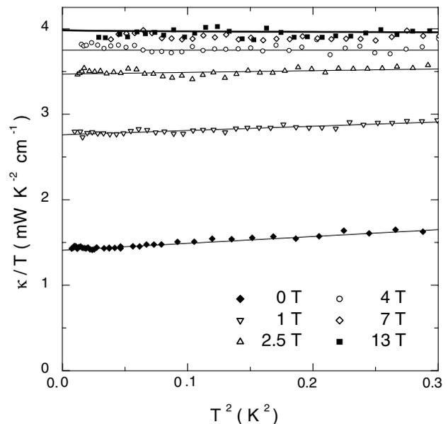
FIG. 2. Thermal conductivity of Tl-2201 for a heat current in the basal plane, plotted as  $\kappa/T$  vs  $T^2$ , at different values of the magnetic field applied normal to the plane. The thin lines are linear fits to the data. The thick line is  $L_0/\rho(T)$  where  $\rho(T)$  is a fit to the resistivity at  $13 \text{ T}$  (see inset of Fig. 1).
