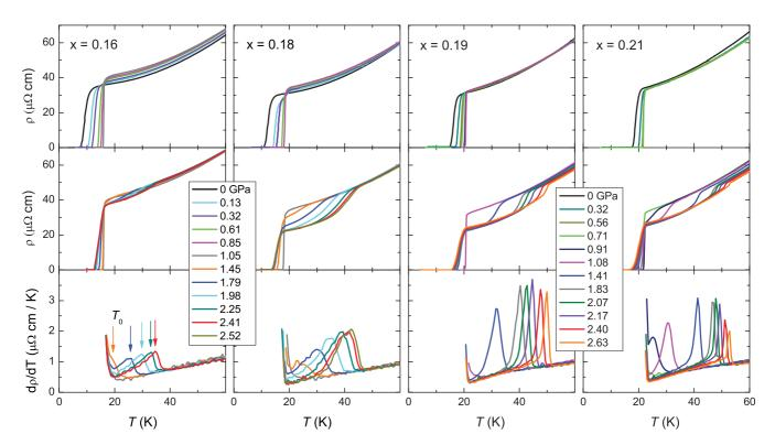
FIG. 2. (Color online) Top and middle: Resistivity of  $Ba_{1-x}K_xFe_2As_2$  with x = 0.16, 0.18, 0.19, and 0.21 (different columns) below 60 K, for pressures as indicated. Bottom: Temperature derivative of the curves in the middle panel. The arrows mark the anomaly at  $T_0$ .
