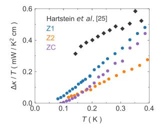
FIG. 7. Field-induced thermal conductivity enhancement at low T for the zone-grown samples, plotted as  $\Delta \kappa / T = [\kappa (H_{\text{max}}) - \kappa (0)]/T$  vs T, where  $H_{\text{max}} = 15$  T for Z1, Z2, and ZC, and 12 T for the sample of Ref. [25] (black diamonds).
