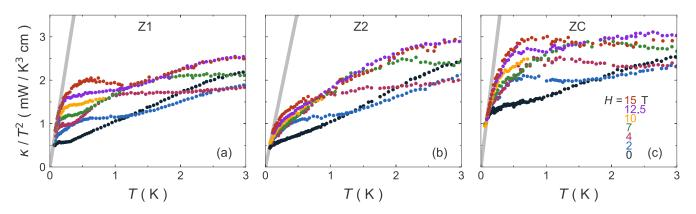
FIG. 5. Thermal conductivity of samples Z1 (a), Z2 (b), and ZC (c) plotted as  $\kappa/T^2$  vs T up to 3 K and for various magnetic field applied perpendicular to the heat current. The gray line in each panel shows the estimated boundary-limited phonon contribution, calculated using Eq. (1) and the appropriate sample dimensions.
