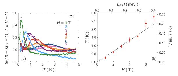
FIG. 6. (a) Normalized difference between two temperature dependencies for the Z1 sample measured at two consecutive magnetic fields, with field applied perpendicular to the heat current. A maximum in the difference (e.g., vertical arrow for 1 T) is observed at a temperature that scales with magnetic field. (b) The temperature of that maximum as a function of magnetic field. All lines are guides to the eye.
