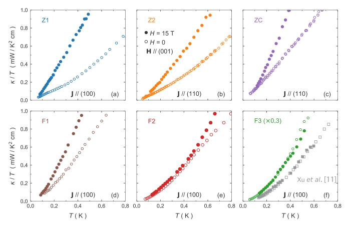
FIG. 2. Thermal conductivity of our three zone-grown (upper panels) and flux-grown (lower panels) samples of SmB<sub>6</sub>, plotted as  $\kappa/T$  vs *T* for H = 0 (open circles) and H = 15 T [full circles; **H**//(001)]. In panel (f), we reproduce the data by Xu *et al.* [11] taken on a flux-grown sample (H = 0, open squares; H = 14.5 T, full squares) and compare them with our own flux-grown sample F3 (multiplied by 0.3).
