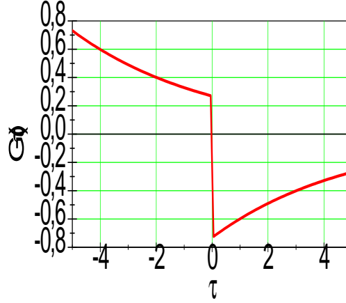
Figure 31-4 \mathcal{G}_0(\mathbf{p}, \tau) for a value of momentum above the Fermi surface.
