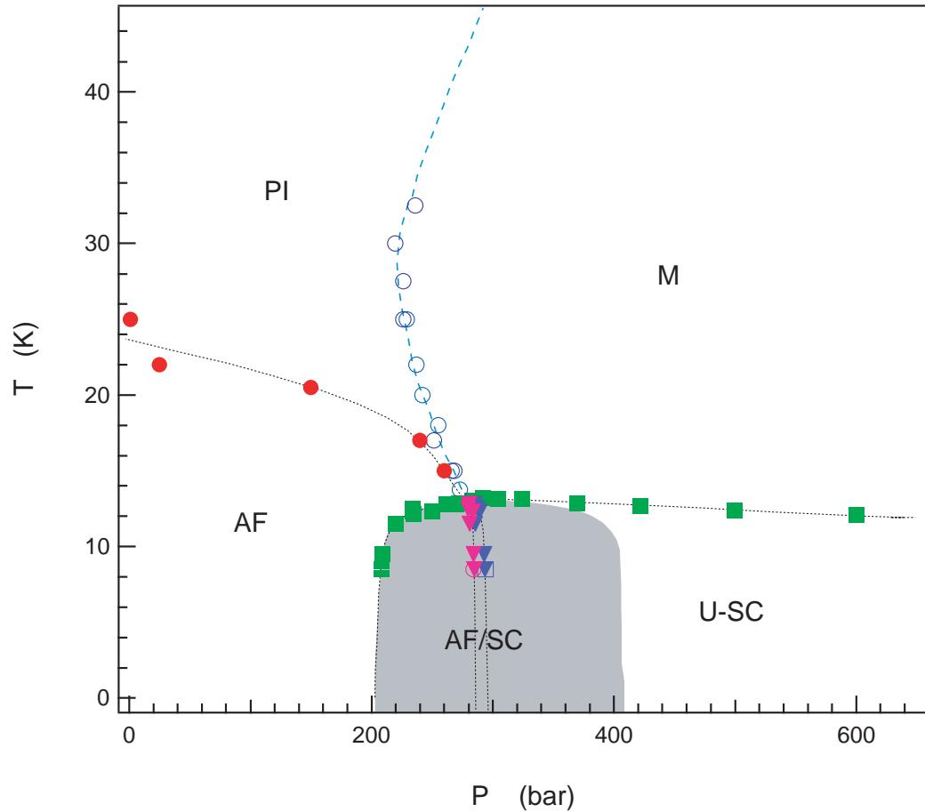
Phase diagram ( $X=\text{Cu}[\text{N}(\text{CN})_2]\text{Cl}$ )
