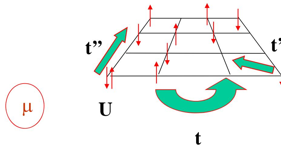
$$H = - \sum_{\langle ij \rangle \sigma} t_{i,j} (c_{i\sigma}^\dagger c_{j\sigma} + c_{j\sigma}^\dagger c_{i\sigma}) + U \sum_i n_{i\uparrow} n_{i\downarrow}$$
