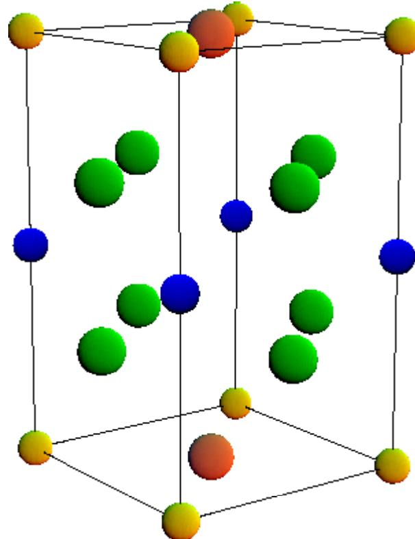
**Figure 1.** The structure of the CeMIn<sub>5</sub> materials. The Ce (Wykyoff position 1a) atoms are yellow, the In(1) (1c) atoms are orange, the In(2) (4i) are green, and the M atoms are blue (1b). Details of the structural parameters can be found in [10]. **Hyperfine interactions in the heavy fermion CeMIn<sub>5</sub> systems** N J Curro
