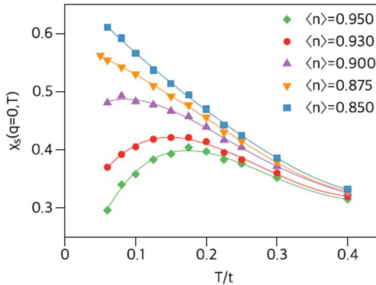
**Fig. 3** Temperature and doping dependence of the  $q=0$  spin susceptibility. At the smaller dopings (larger filling  $\langle n \rangle$ ),  $\chi_s(T)$  exhibits a peak in the temperature dependence indicating the opening of a PG
