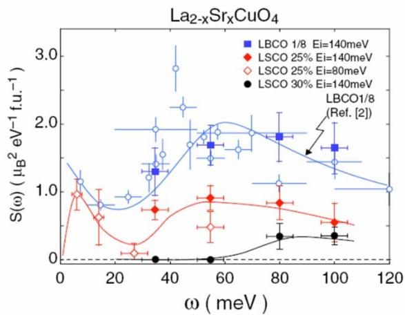
FIG. 3 (color online).  $\mathbf{Q}$ -integrated dynamic structure factor  $S(\omega)$  which is derived from the wide- $H$  integrated profiles for LBCO 1/8 (squares), LSCO  $x = 0.25$  (diamonds; filled for  $E_i = 140$  meV, open for  $E_i = 80$  meV), and  $x = 0.30$  (filled circles) plotted over  $S(\omega)$  for LBCO 1/8 (open circles) from [2]. The solid lines following data of LSCO  $x = 0.25$  and 0.30 are guides to the eyes.
